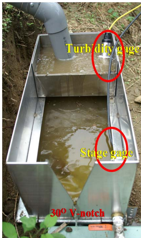
Fig. 11 V-notch weir installed with a pressure-type stage gauge to record the water stage and turbidity gauge.
