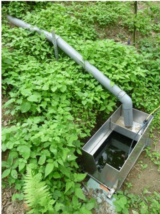
C. Runoff and soil losses monitoring plot was set up at this site.
